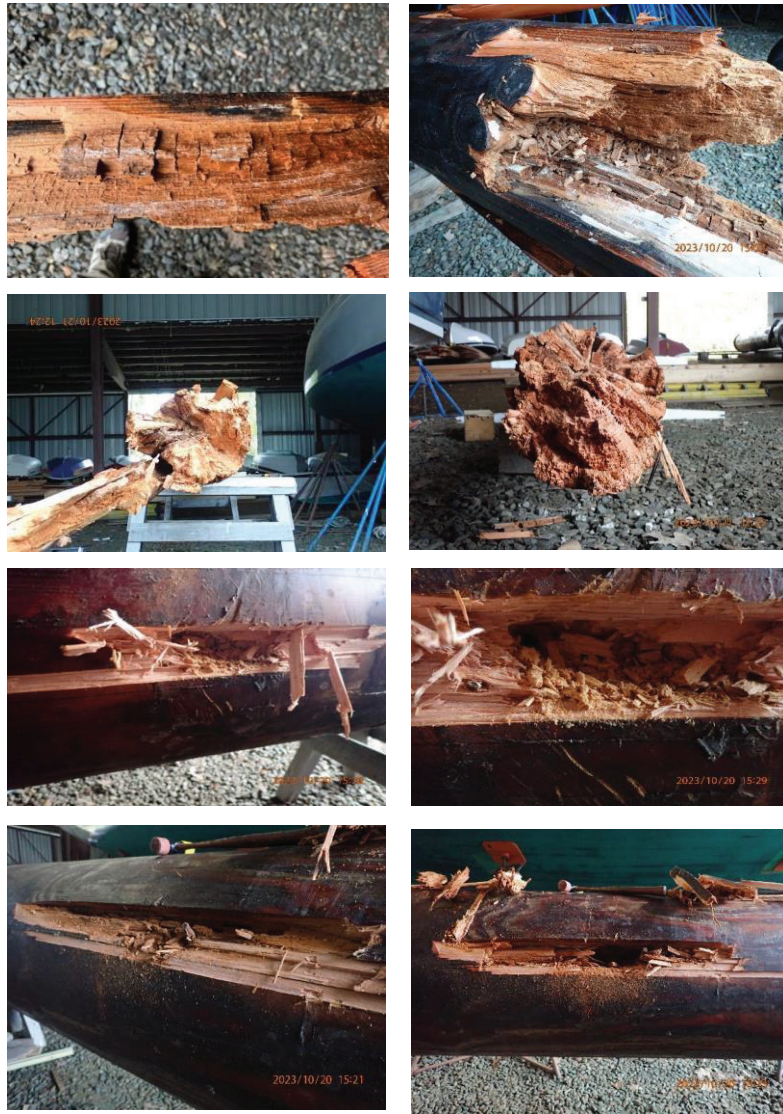
Figure 5 – Photos depicting brown rot decay at the breakpoint and various locations along lower portion of the broken mainmast.
