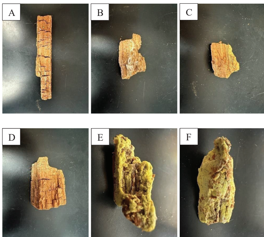
Figure 6. Sections of Douglas-fir decayed mast showing brown-rot and yellow fungal mycelia. A) breaking point 47-48; B) upper breaking point; C) breaking point 36; D) breaking point 28; E-F) breaking point 43.
