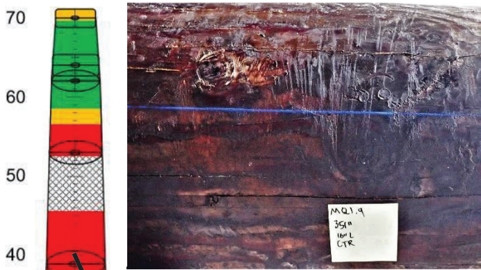
Figure 39 – Check Number 1.9 (35" length). Probing revealed soft wood, penetrating into the center without resistance.
