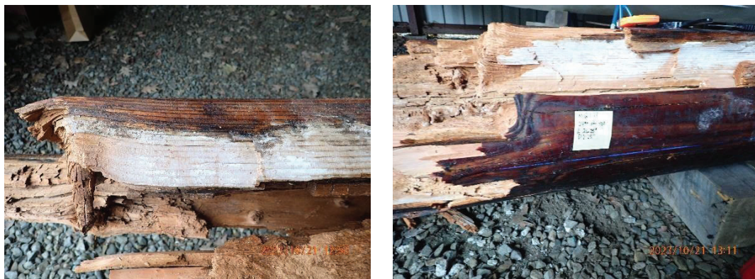
Figure 65 – White mycelial matting observed along check surfaces
