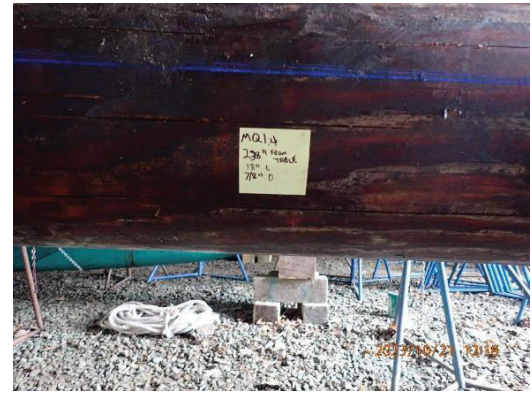
Figure 24 – Check Number 1.4 (18" length x ¾" depth). Probing did not reveal soft wood.
