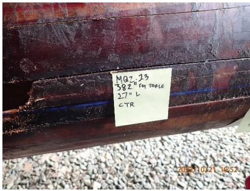
Figure 43 – Check Number 2.23 (27" length). Probing revealed soft wood, penetrating into the center without resistance.
