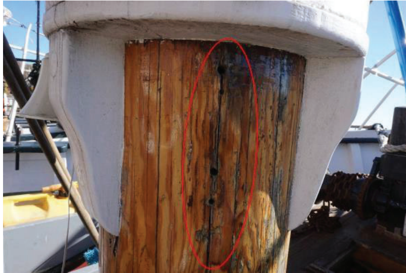
Figure 14 - Foremast rot identified during survey, November 23, 2022. (Source: Maine Design report of survey)
