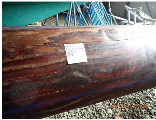
Figure 26 – Check Number 2.14 (35" length x ½" depth). Probing did not reveal soft wood.
