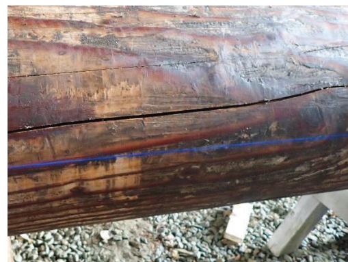
Figure 10 – Check Numbers 2.3 (46" length x ½" depth) and 2.4 (33" length x ½" depth). Probing did not reveal soft wood.
