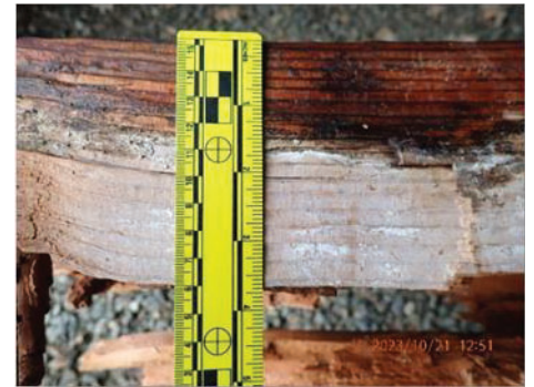
Figure 4 – Deep check present at breakpoint depicting wide growth rings, inadequate penetration of slush, and remnants of mycelial matting.
