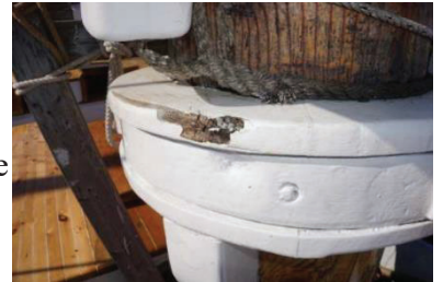
Figure 13 - Rot in foremast boom saddle found during survey, May 5, 2022, (Source: Maine Design report of survey)
