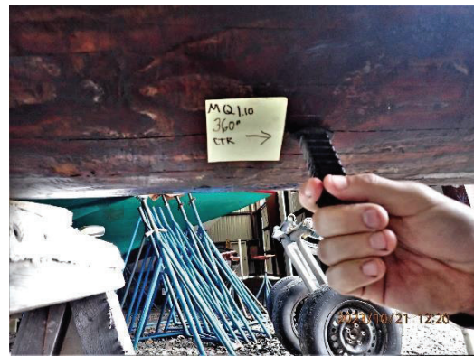
Figure 42 – Check Number 1.10 (18" length) Probing revealed soft wood, penetrating into the center heartwood without resistance.
