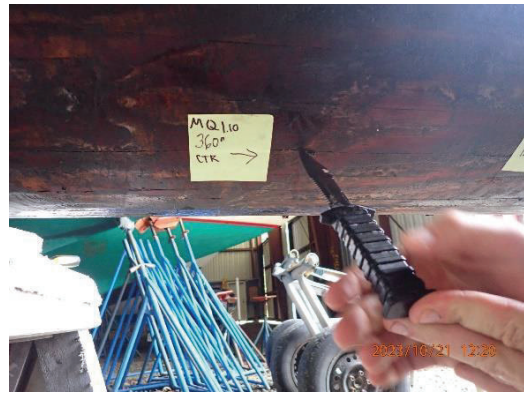
Figure 40 – Check Number 1.10 (18" length) Probing revealed soft wood, penetrating into the center without resistance.
